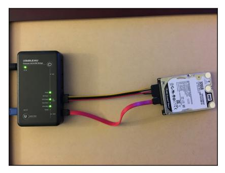
6. With the physical write blocker in place, the suspect drive is now ready for imaging. In this example, the freeware application FTK Imager will be used. FTK Imager requires administrator privileges to run. Open the executable and the following screen will appear:
