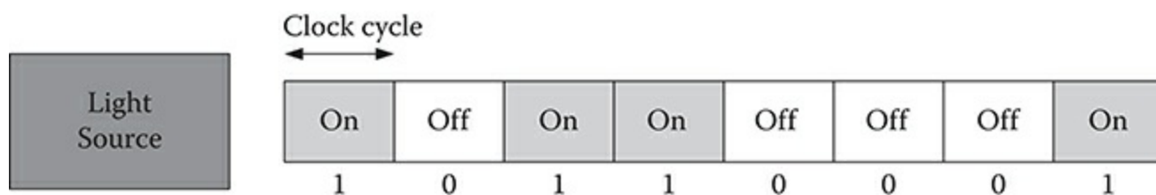
Figure 4.2 On/off digital signaling.
