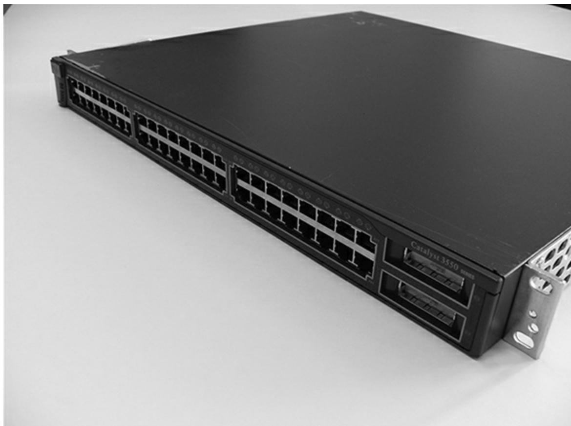
Figure 3.14 An Ethernet layer 3 switch.
