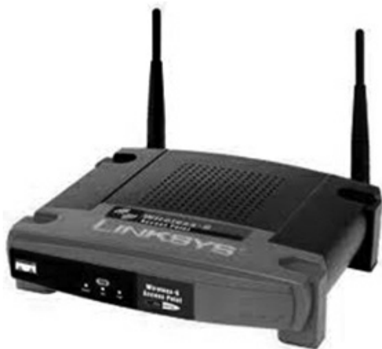
Figure 8.4 Wireless access point. (Source: linksys.com .)
