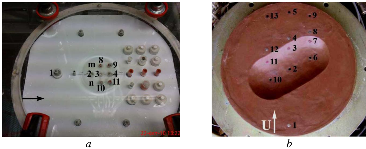
Fig. 2. Ensembles of the wall pressure fluctuation sensors on streamlined surface of the spherical cavity (a) and the oval dimple (b)
